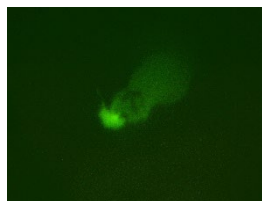
After Cryptolyte® Remnants of Crypto oocyst 1000x Epifluorescence
